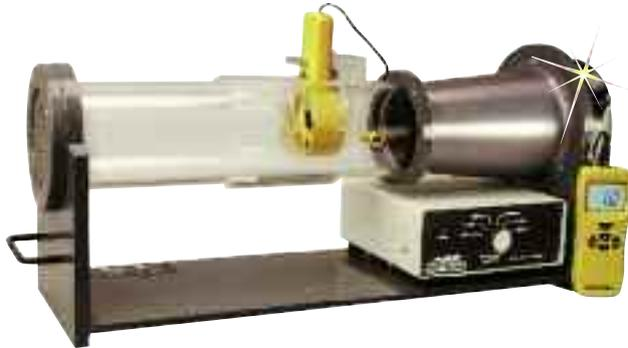
Figure 2 –Benchtop Calibration Wind Tunnel (Omega Engineering, Inc.)
