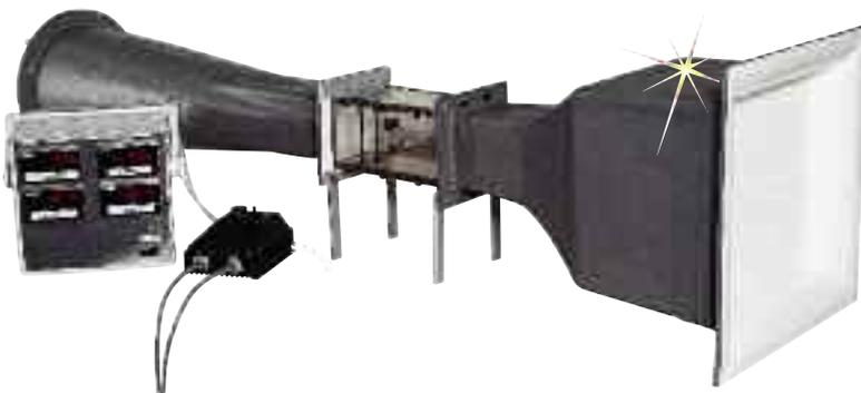
**Figure 1** shows a typical benchtop wind tunnel (Omega Engineering, Inc., Stamford, CT). The transparent test chamber can be seen in the center. A fan on the left pulls air into the square opening on the right where a fiberglass honeycomb filter produces a uniform stream that is then shaped by the duct leading to the air chamber. This unit can be used for either calibration or air flow studies.
