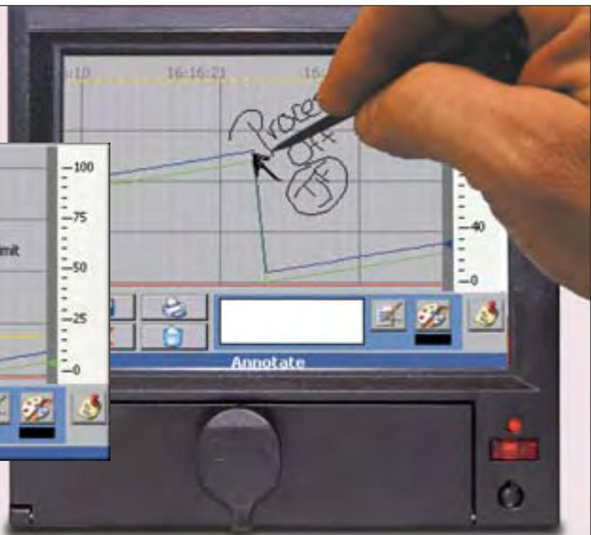
The innate feature of handwriting notes and comments on the chart of paper recorders had been lost with the onset of video graphic recorders until the arrival of the RD8300. Using the high-resolution touch screen interface and the integral stylus you can once again make notes or comments directly on the chart. This on-screen annotation is stored within the data file directory and can be recalled and displayed on the recorder or in Exhibitor Software.
